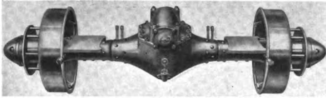
Model W-5 Sheldon worm-gear axle for 5-ton trucks
